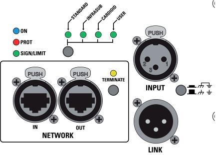
2) Pressing it with the unit ON you can select the DSP PRESET. The selected PRESET is indicated by the corresponding LED:
