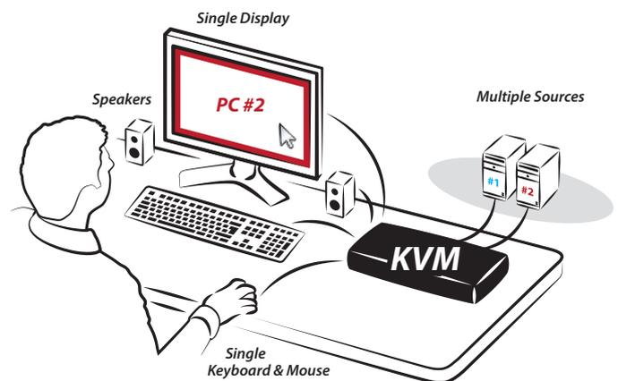
HSL Single-Head 2-Port KVM Switch System Diagram
