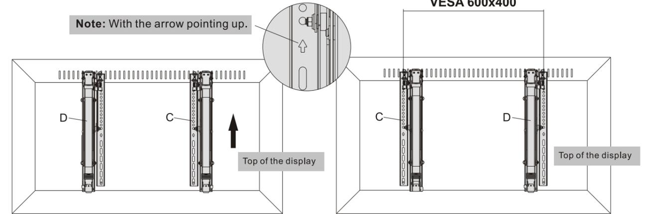
For VESA 600x400, the positions of "D" and "C" are exchanged.
