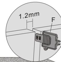
**Note:** Use the plastic locking piece to measure and keep a 1.2 mm gap between displays.
