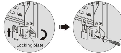
Turn the locking plates downward to fasten the wall plate and tighten the screws to secure.
