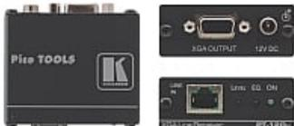
The PT-120xl is an extended range twisted pair receiver for computer graphics video signals. It converts a twisted pair signal from a WP-110 transmitter (or other compatible Kramer transmitter) to a computer graphics signal
