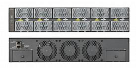
NETGEAR M4300–96X (empty switch) is a NETGEAR modular managed switch chassis used for large AV over IP deployments. It can be populated with module units in increments of 8 10GBASE–T, 8 10GBASE–X (fiber SFP+) ports or 2 QSFP+ ports.
