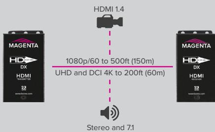
The HD-One DX series is available in HDBaseT and extended range variants in a compact form factor for the transmission of HDMI 1.4 signals including 1080p, 3D, UHD/4K and 4K DCI. Together, the HD-One DX series has full audio support including LPCM 7.1CH, Dolby, TrueHD, Dolby Digital Pluys and DTS-HD.
