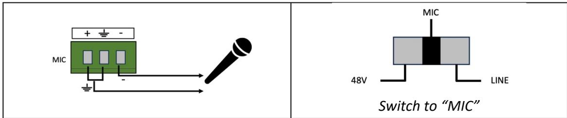
2) Balanced connection: "+" connects to positive, "-" connects to negative and "⊥" connects to ground.
