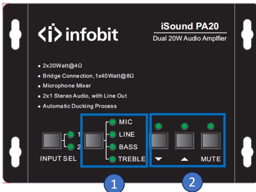
For example, to turn up the line volume, you should select the “LINE” first, and then press the button “▲”.
