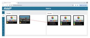
③ Left-click the Encoder and drag it to multiple Decoders, then release the mouse to realize one-to-many switching.
