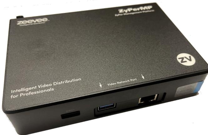
Installations may require a ZyPer Management Platform (ZMP). This device controls the operation and manages the connectivity between endpoints. The management platform is a hardened controller node that must reside on the same logical network as the ZyPerUHD60 Encoders and Decoders. It runs a ZeeVee application as its sole function. The application presents an API to potential third party management platforms as well as hosting its own management application.
